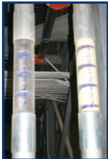
**PRODUCT SEGREGATION:** Diamond V installed Cablevey tubular drag conveyors to allow complete cleanout of one product without any changeover time.
